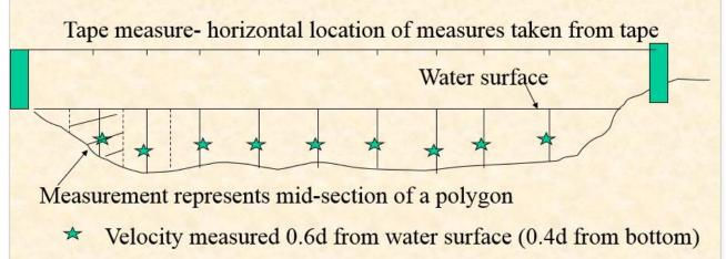
Record x value (tape distance), y value (total depth at measurement site, and velocity at 0.6d
